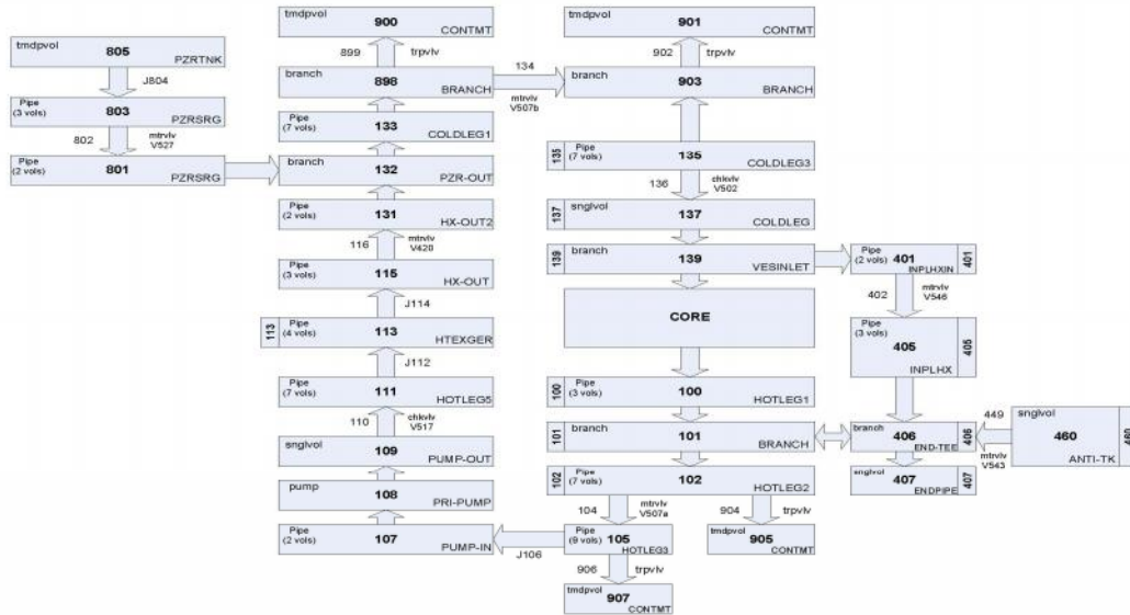
Figure 2: MURR RELAP/SCDAPSIM Nodalization of the MURR Pressurized Primary Cooling System.
